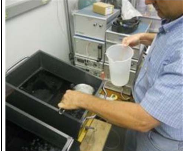
2. Collecting Samples/Fibres from the Slosh Box.
