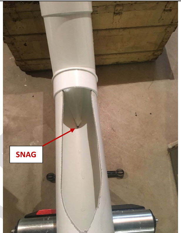
Photo A.4 –Snag Left by Previous Tests Prior to Commencing a New Test to be Removed.
