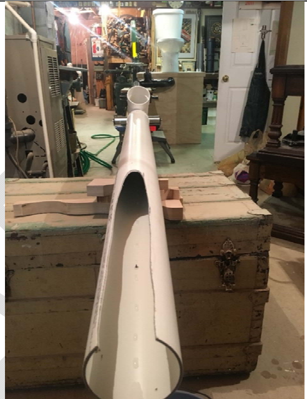
Photo A.2 - Galvanized Screws Used as Snagging Obstruction
