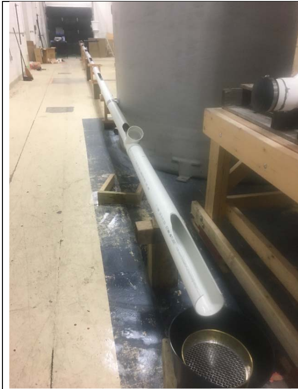
Photo A.3 – The Drain Line and Sieve Used to Capture the Flushed Product.
